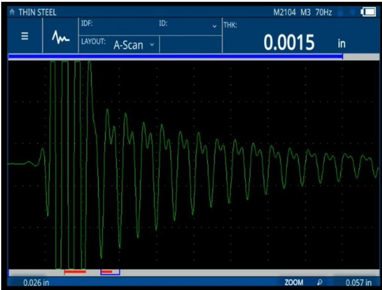
72DL PLUS gauge measures a thin steel sheet (0.0015 in. or 0.0381 mm) using the M2104 (125 MHz) transducer
